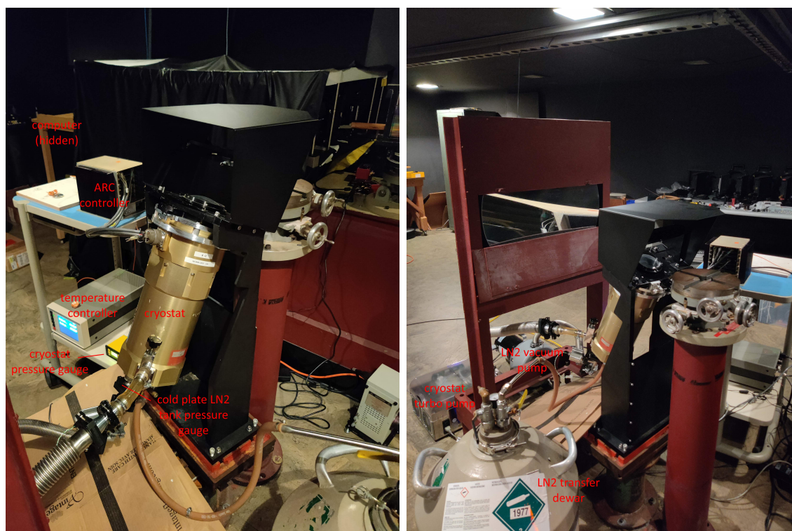
Figure 3.1: ODESSA set up in the Coudé room of the McKellar Spectrograph, with major components labelled. The ARC controller and temperature controller connect directly to both the cryostat and the computer (out of view). The two vacuum pumps connect to different parts of the cryostat, where they are both monitored by pressure gauges. The fill tube of the LN2 transfer dewar is used for both of the cryostat’s LN2 tanks.
