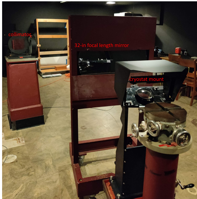
Figure 2.2: The 32-in arm of the McKellar Spectrograph. Light from the collimator (left) is dispersed off a diffraction grating (not shown), reflected off the 32-in-focal length mirror (centre), then redirected onto the focal plane by a flat mirror on the detector mount (right).
