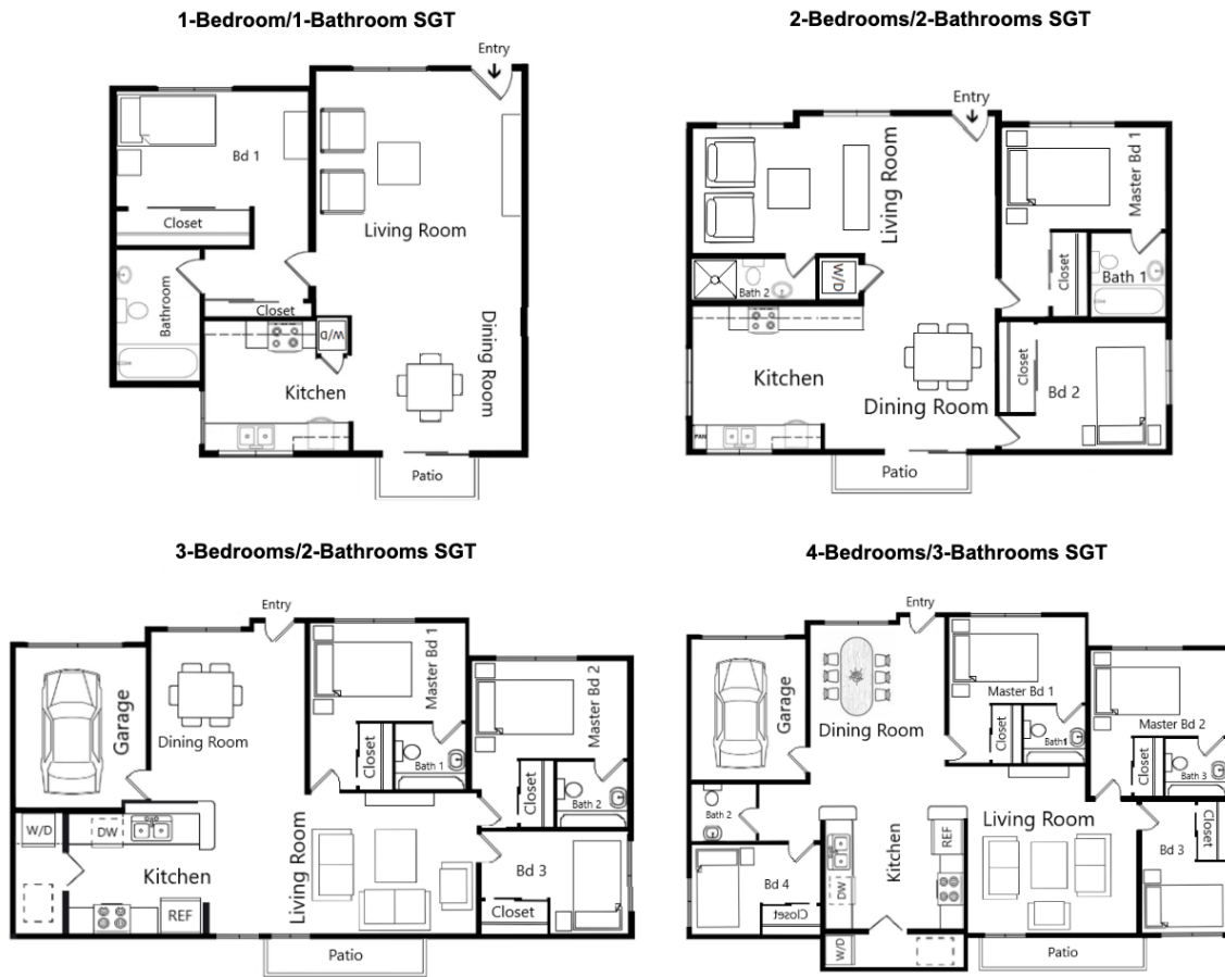
Figure 3.4: 1 to 4 bedroom SGT floor plans.
