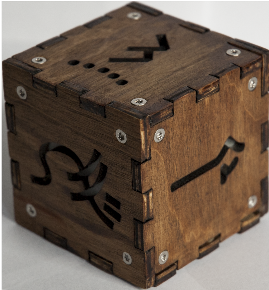
Figure 4.7: Final wooden form for Transcode control interface. Note the hardware countersunk and flush with cube faces as well as stained finish.
