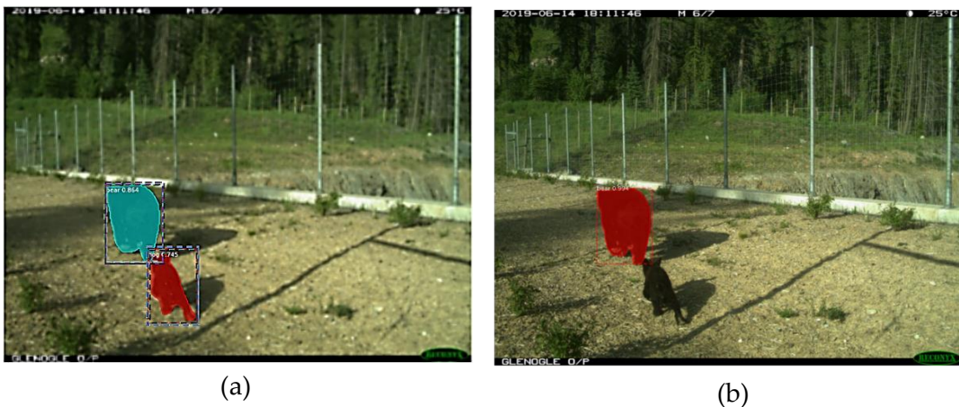
Figure 3.5: Effect of IoU threshold on the animal detection using the deformable Mask R-CNN. (a) High threshold scenario (two bounding boxes generated for each detected bear). (b) Low threshold scenario (only one bear detected, with a single bounding box).
