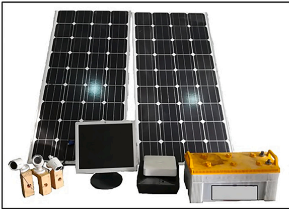
Fig. 1. The video recording components including solar panels, cameras, monitor, DVR, and UPS used for recording traffic data on a 200 m road section.
