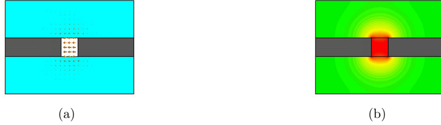
Figure 5.6: Electric field distribution of the terahertz mode of in metallic slit - silicon structure. (a) Field vectors at 2THz, (b) Field magnitude at 2THz.
