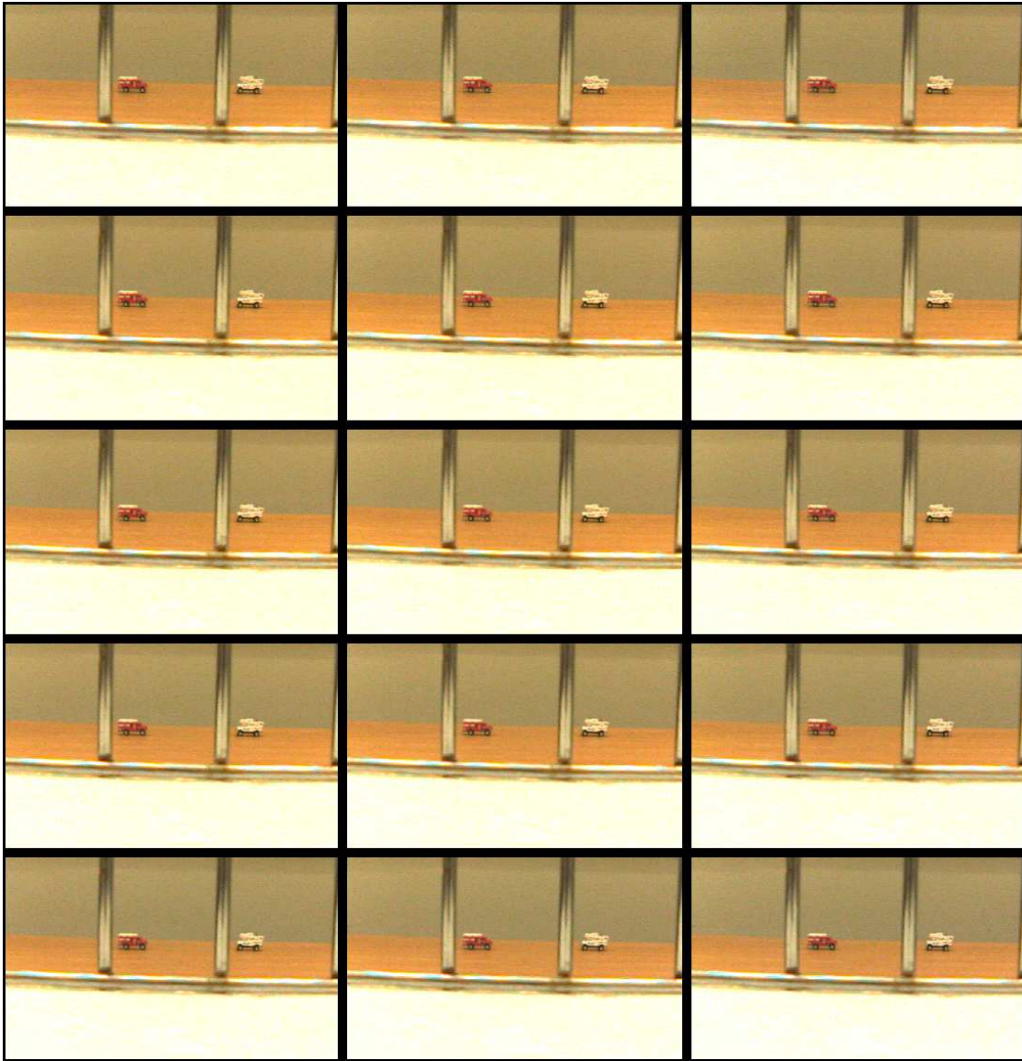
Figure 3.11: The 20th frame of the LFV corresponding to the central 15 sub-apertures ( n_x = 4, 5, 6 and n_y = 3, 4, \dots, 7 ). The white truck is the object of interest; the red truck is the moving interfering object; the fence is the static interfering object.
