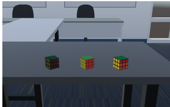
Figure 5.3: Three Rubik’s Cubes in the Virtual Reality Environment: Photogrammetry-Based (Left), CAD Model (Center), Gaussian Splat-Based (Right)
