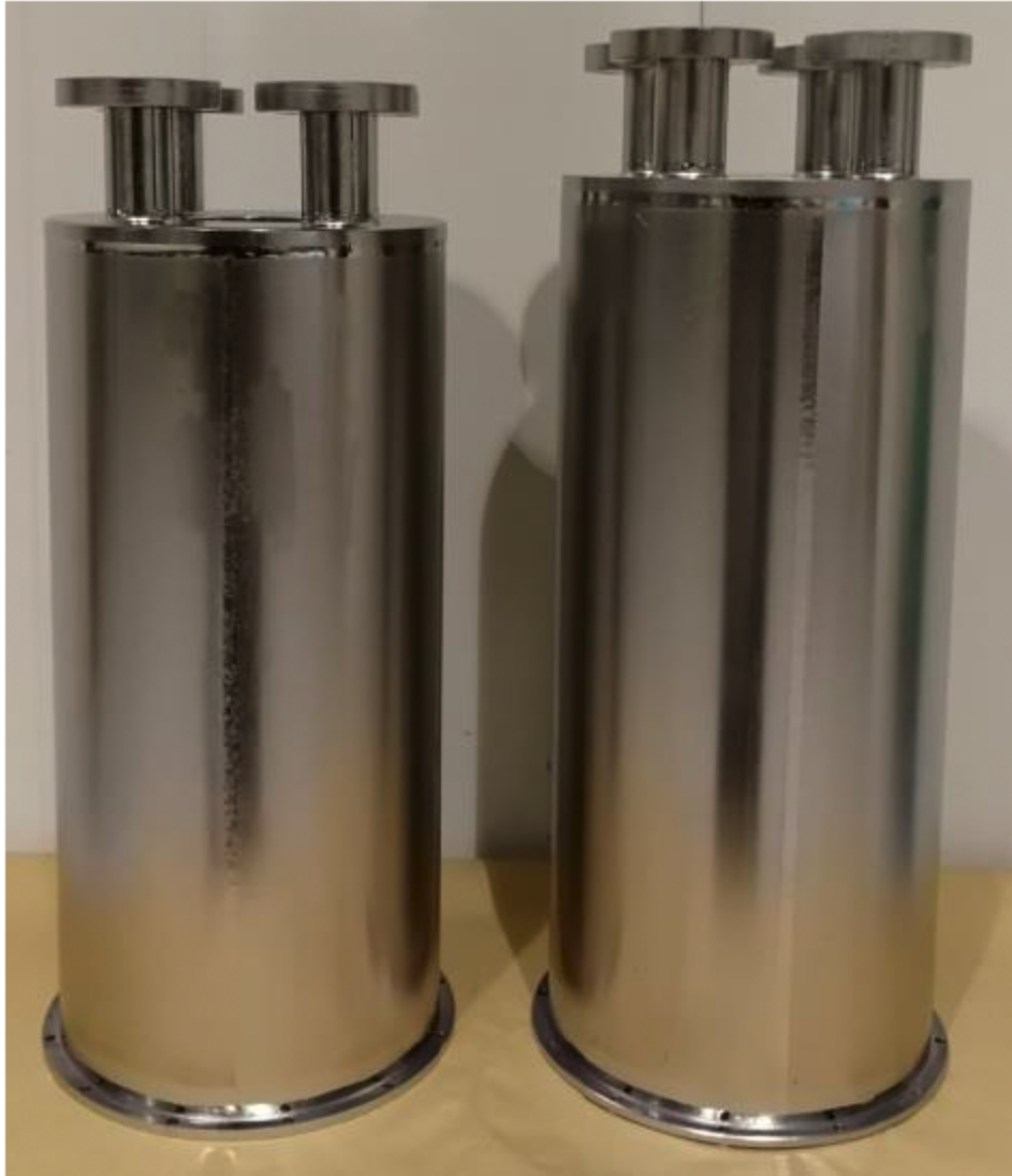
Figure 2.1: Photo of two coaxial cavities. Photo courtesy of [12].
