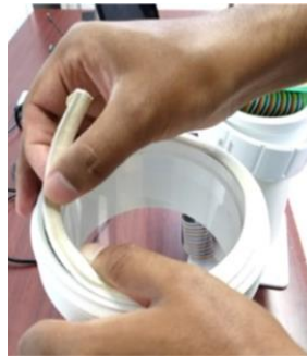
FIGURE 38 WEATHER STRIP SEALING, FROM SMT REPORT
