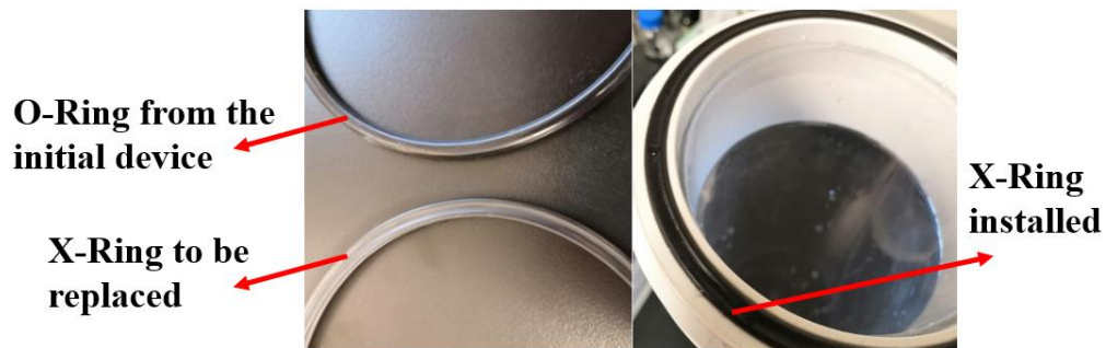
FIGURE 43 COMPARISON BETWEEN O-RING AND X-RING
