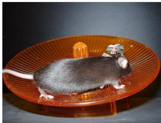
Figure 3: Experimental setup for measuring the acceleration of mouse gait.
