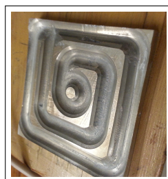
Figure 5.4: Aluminum plate ridges that improve the contact between the ceramic heater and the fin system base.
