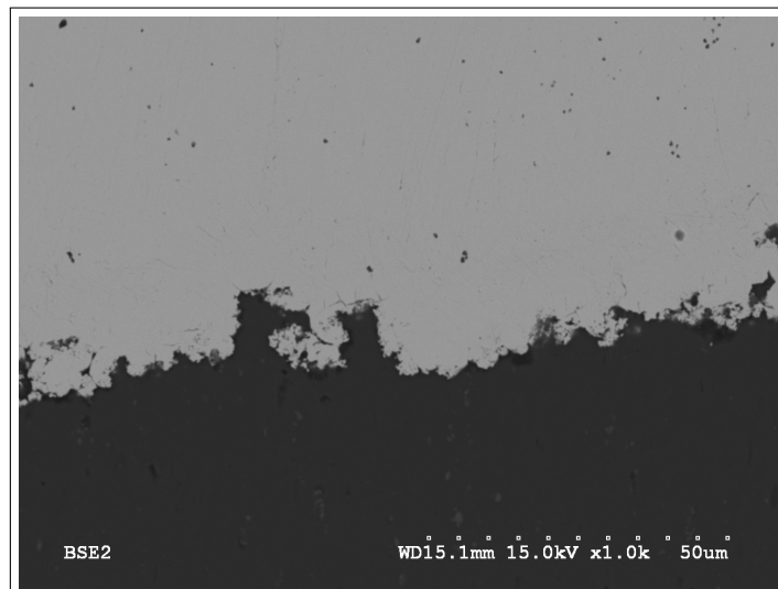
Figure 4.7: Detailed features of the gold-aluminum interface for the 0.5 mm thick sample shown for the same scale as figure 4.5 (a).
