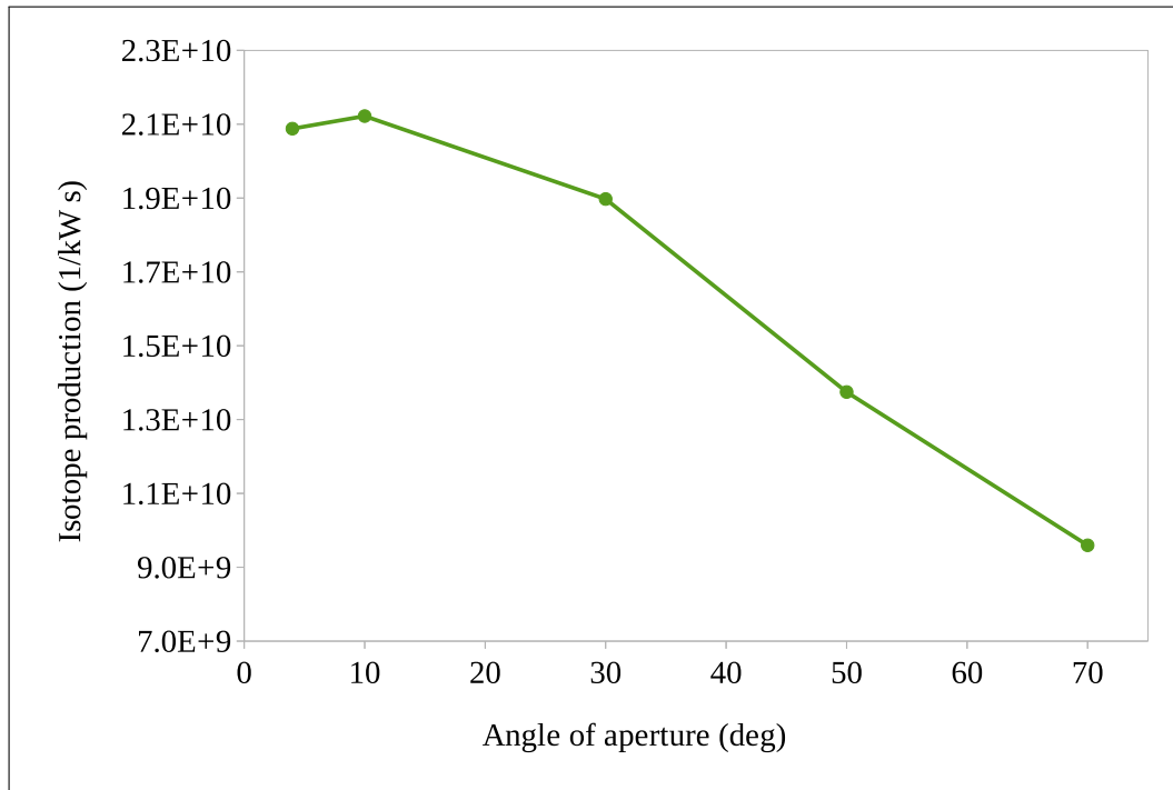
Figure 2.9: Isotope production of a converter with different trench apertures with a fixed effective thickness of the converter coating.
