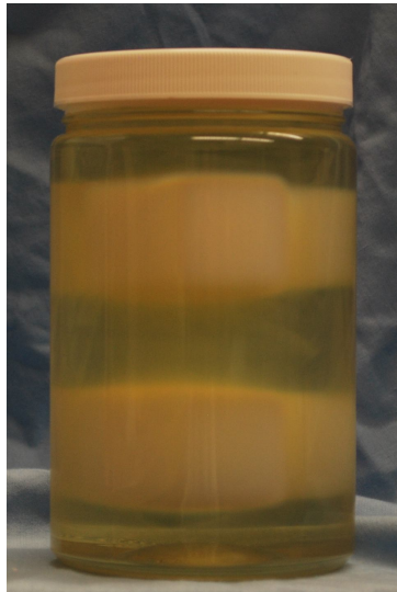
Figure 1.9: A polymer gel dosimeter exposed to ionizing radiation at the top and bottom of the container (white regions). Gel dosimeters are truly 3D radiation measurement tools that show great promise for complex treatment verification.
