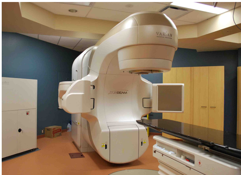
Figure 1.4: A LINAC in modern RT used to deliver external beam therapies. Similar to the CT simulator, lasers mounted on the treatment room walls to the left and right of the LINAC and on the ceiling (not visible in figure) are used for patient positioning at each day of treatment.
