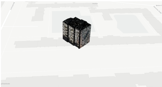
Figure 3.21: The object is offset on the map when loaded into the scene combined with Babylon and Mapbox.
