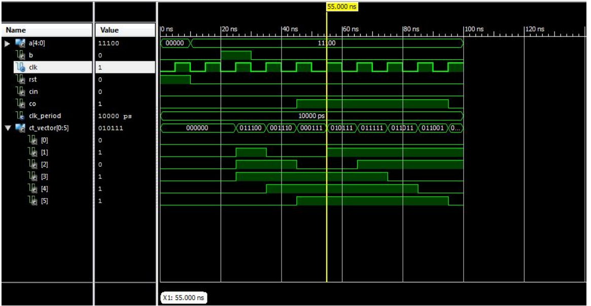
Figure 5.1: Resultant wave from for systolic array, m = 5 and k = 2
