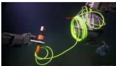
(a) ROPOS (Remotely operated platform for ocean science) delivering seismometer to seafloor.
