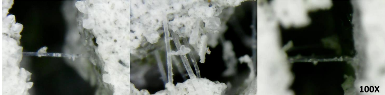
Figure 4-2: Micro fiber crack bridging observed using optical microscopy
