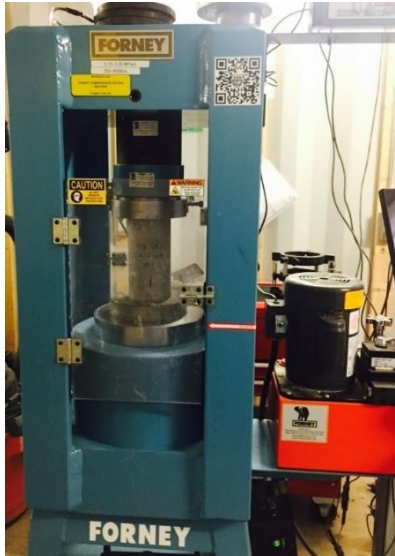
Figure 3-2: Forney Compression Machine Used for Determination of Compressive Strength
