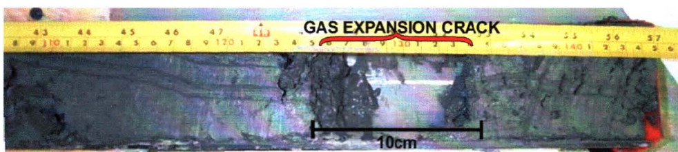
Figure 2.6. Photograph showing the effect of gas expansion on the surrounding sediments. The gas expansion crack is ~10 cm in this case.
