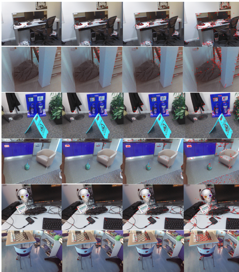
Figure 2.2: Illustrations of image feature extraction using SURF descriptor. Red dots represents the location of (from left to right:) 10, 50, 100 and 300 SURF features of (from top to bottom:) office, stairs, fire, pumpkin, heads and chess scenes.
