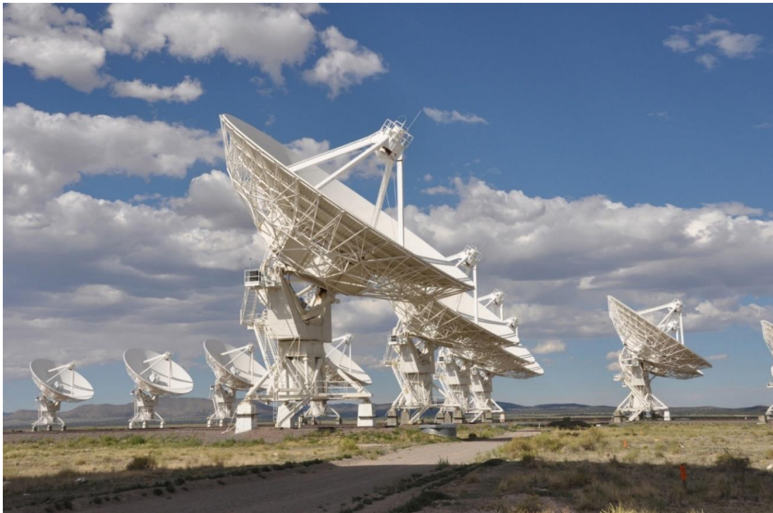
Figure 1.1. The Very Large Array in New Mexico, which operates mostly at cm-wave frequencies. The 28 antennas are of 25 meter diameters. Credit: NRAO.
