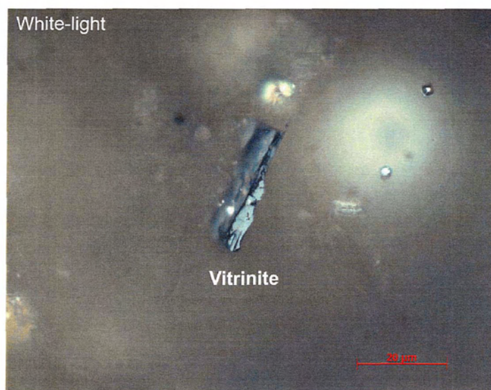
Figure 7.2. The white light microscopy (reflected light) of a typical sediment sample showing a low reflectance particle of coal maceral (vitrinite) originating from the surrounding outcrops in the study area. (for details on methodology see Chapter 1.7.3.4 and 8.2.2).
