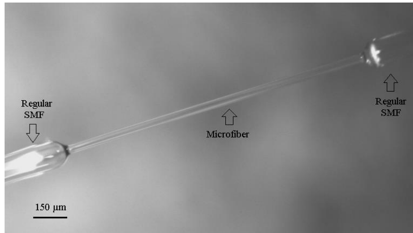
Figure 7.2 Splicing of the microfiber between two standard SMFs prior to grating fabrication in order for improve handling of the fiber during modulated index inscription
