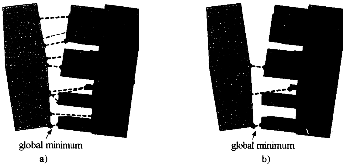
Figure 4.12. Example of the GA using a) sharing and b) deterministic crowding on the battery and fixture case.
