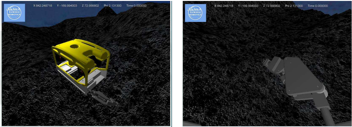
Figure 7: Snapshots from the Visualization tool. The left image is a third party view and the right image is the camera view.
