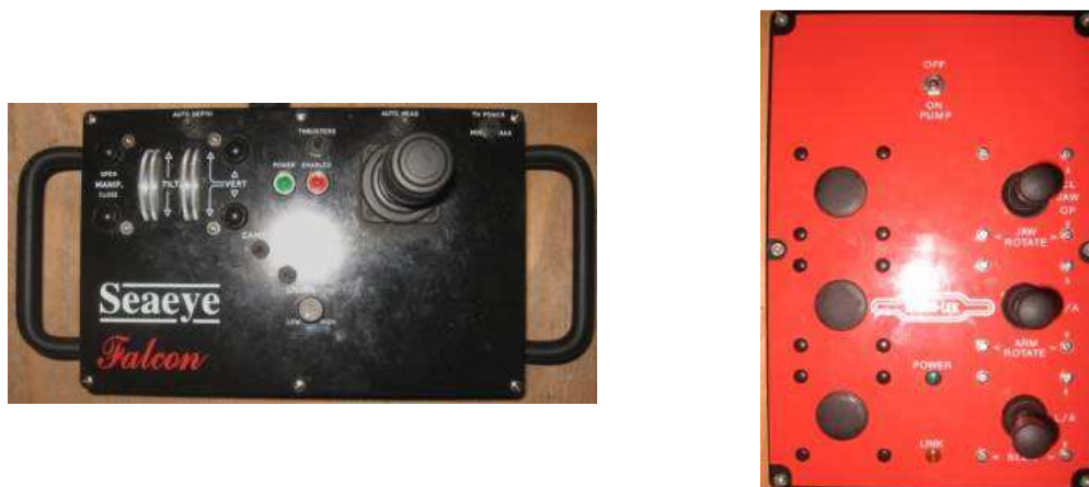
Figure 9: On the left is the Falcon™ HCU that allows the human pilot to operate the vehicle. On the right is the HCU of the HLK 43000 underwater manipulator. By pushing/pulling the corresponding joystick on the manipulator HCU, individual joints can be moved. Currently, the manipulator HCU allows commanding only one joint motion at a time.
