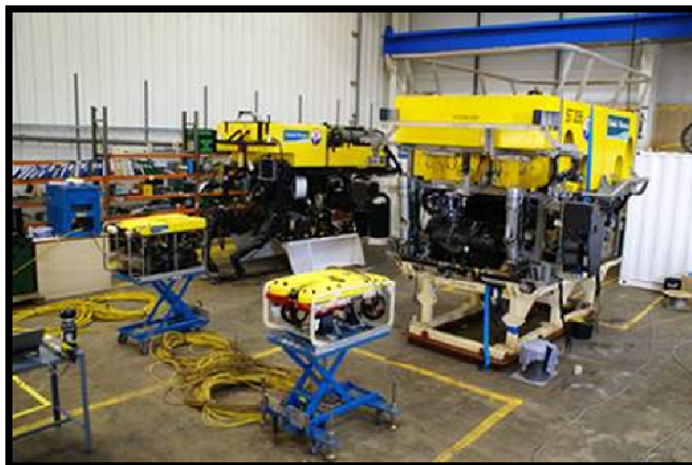
Figure 3: The difference in size can be seen between a work-class ROV and an inspection-class ROV. Image courtesy of http://oceanscan.net .
