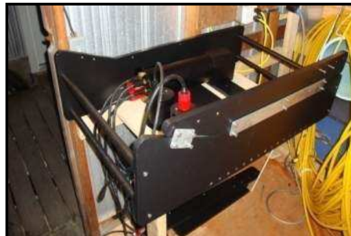
Figure 12: A series of water-proof, pressure proof sensor canisters for each sensor were designed. The modular design allows the location optimization of each sensor on the new navigation skid in order to minimize magnetic interferences mostly due to the onboard thrusters.
