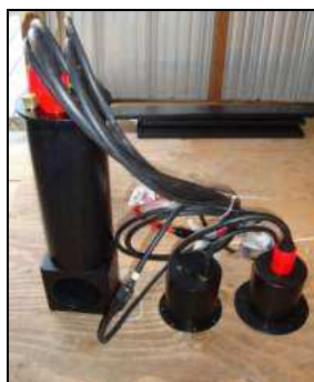
Figure 12: A series of water-proof, pressure proof sensor canisters for each sensor were designed. The modular design allows the location optimization of each sensor on the new navigation skid in order to minimize magnetic interferences mostly due to the onboard thrusters.
