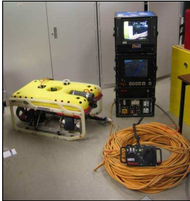
Figure 7: Inspection-class SeaEYE Falcon™ ROV systems. Due to their one to one ratio between its weight and trust, these systems are commonly used in industry. This system was used as a test-bed for the experimental portion of the current work. Image courtesy of [43].
