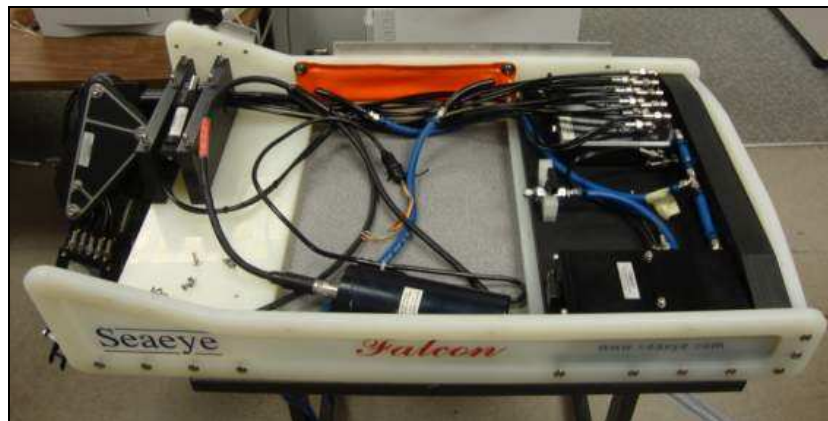
Figure 7: Inspection-class SeaEYE Falcon™ ROV systems. Due to their one to one ratio between its weight and trust, these systems are commonly used in industry. This system was used as a test-bed for the experimental portion of the current work. Image courtesy of [43].
