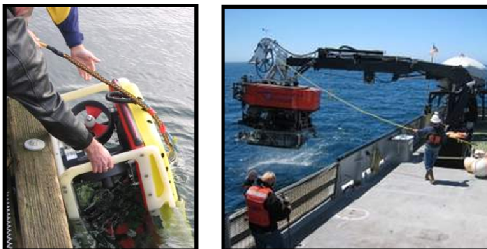
Figure 4: On the left, a work-class ROV is being hand-deployed in the water from a pier. On the right, an inspection-class ROV is being deployed by a crew with a crane attached on the surface vehicle. The image on the right is courtesy of http://polartrec.com .
