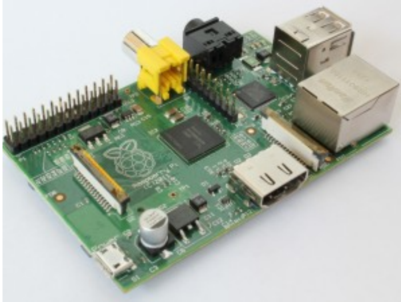
Figure 2.14: A photo of the Raspberry Pi (Model B, Rev 2) Single Board Computer [35].
