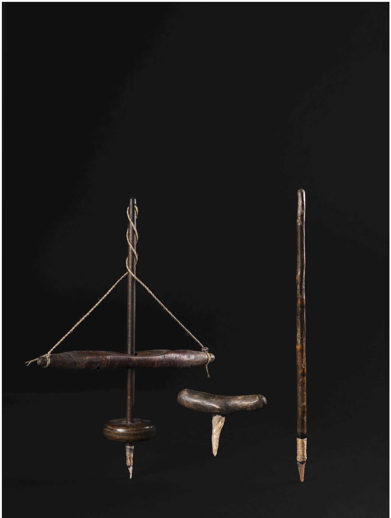
Fig. 4. Reconstructed drills Flint (original), wood and rope (contemporary) L 10.5–34 cm, W 0.6–25.5 cm | Gift of Felix Burian and Erich Friedman, Tel Aviv | IMJ 87.136.139, 140, 142 Photo © The Israel Museum, Jerusalem by Elie Posner.
