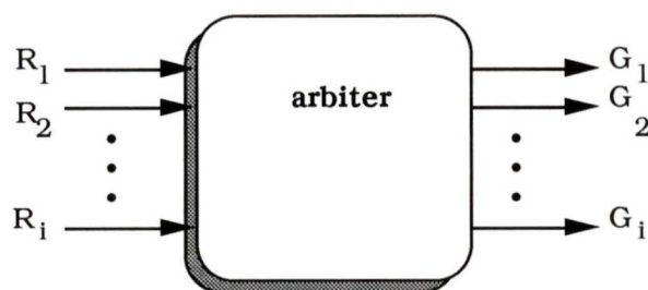
Figure 5.7 Black box representing the mutual exclusive function of the arbitration procedure.
