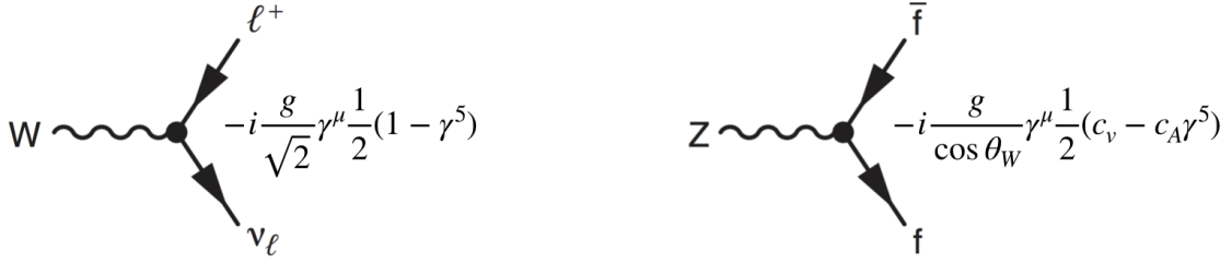
Figure 2.3: Three point vertices for the electroweak bosons and their coupling strengths. c_V is the vector coupling, c_V = T_3 - 2Q \sin^2 \theta_W and c_A is the axial-vector coupling c_A = T_3 . Taken from [23].
