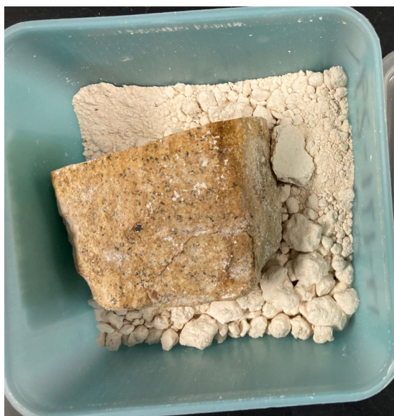
Figure 2.1: A plastic tub containing the core catcher of core 29 of hole 17-171 (17-171-29-CC), which contains hyaloclastite (one large chunk) and carbonate (very friable and broken into smaller pieces; Shipboard Scientific Party, 1973e). The footprint of the tub is about 10 cm x 10 cm.
