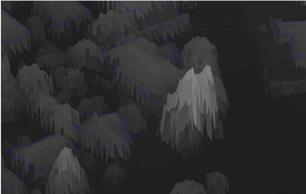
Figure 12 – The resulting DSM at study site #1, oriented at an oblique angle and in a northwards ( \sim 18^\circ ) direction.
