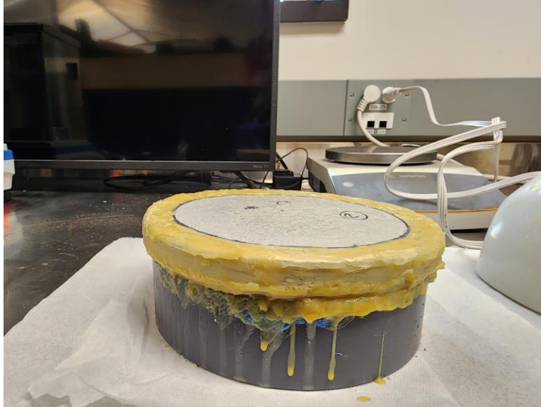
Figure 18. Mortar Specimen Coating with Test Dish
