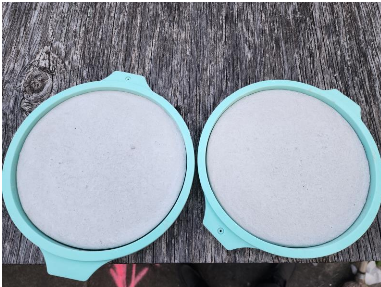
Figure 17. Mortar Specimen Preparation for Water Vapor Permeability Test
