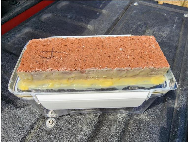
Figure 16. Brick Specimen for Water Vapor Permeability Test
