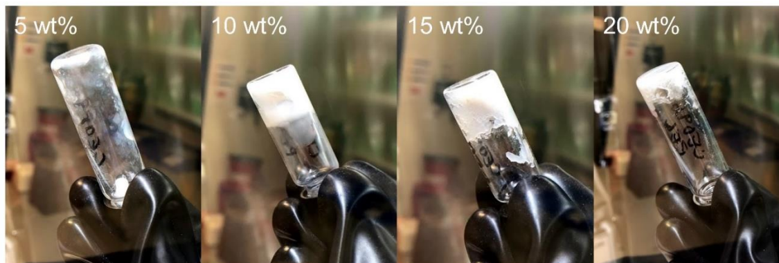
Figure S3.6 Photos showing visual comparison of PEG 205 - b -PFTMC n micelle solutions (target DP n = 40, target block ratio = 5:1) prepared via PI-CDSA in 20 vol% DCM/MeCN at 5–20 wt%.
