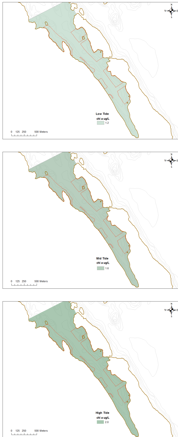
Figure 18: Maps showing the predicted chlorophyll- a concentration in Trevenon Bay at three tidal heights (low tide, mid tide, and high tide). The darker the green color, the higher the chlorophyll- a concentration. The red polygons mark the locations of the shellfish farms.
