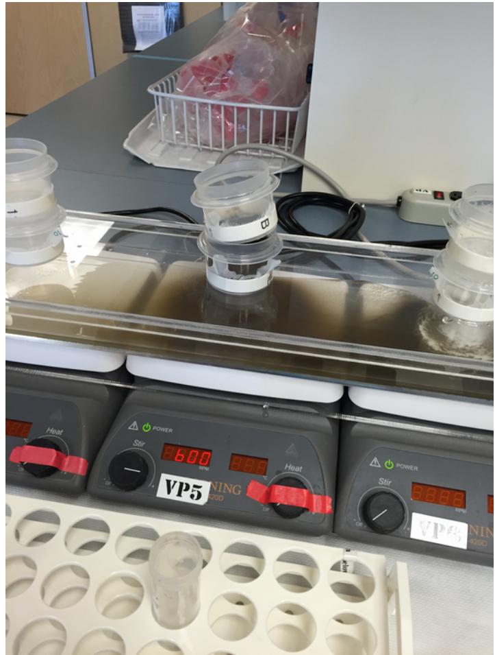
Figure 3.1. Sieving apparatus designed by Vera Pospelova (University of Victoria) for palynological application. Nylon sieves are attached to the open bottom of the plastic food containers as shown, and stacked with the coarser sieve on top. A stirring rod on the lower sieve is spun by a magnetic stirrer. Water and fine sediment is collected in the reservoir which is allowed to drain. RO water is fed into the system gradually until the water coming out of the lower sieve is clean and the material on that sieve is retained.
