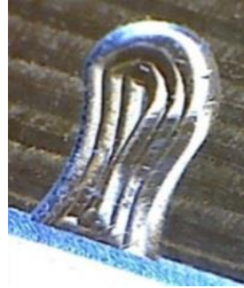
Figure 5-16 : Machined pocket with tool diameter 0.794 mm
