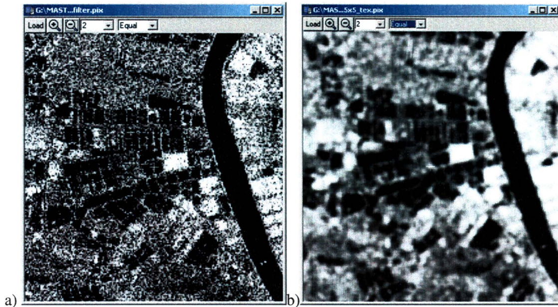
Figure 6.11 a) Original F4 image of May 7, 2001 b) 5x5 Mean Texture image of May 7, 2001
