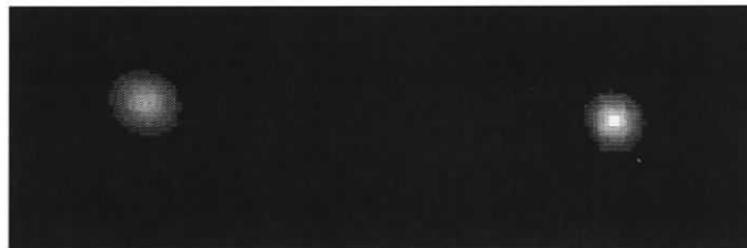
Figure 5.8: Measured distorted image (left) with the respective Type 1 system corrected image (right)
