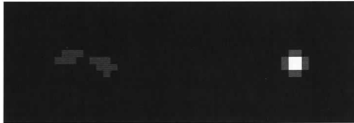
Figure 5.7: Simulated short exposure distorted image (left) and the Type 1 system corrected image (right)
