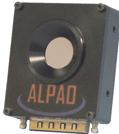
Figure 26 - The ALPAO DM52 deformable mirror used in the optical tweezer. The mirrors 52 actuators are addressed using serial communication with between a PC DAQ card (Adlink Powerdaq 64) and DM drive electronics (ALPAO DE64).
