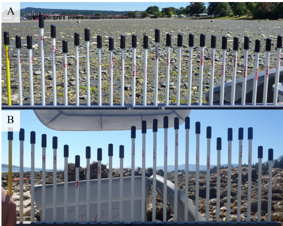
Figure 5. Profile gauge deployed on low complexity (A) and high complexity (B) surfaces.
