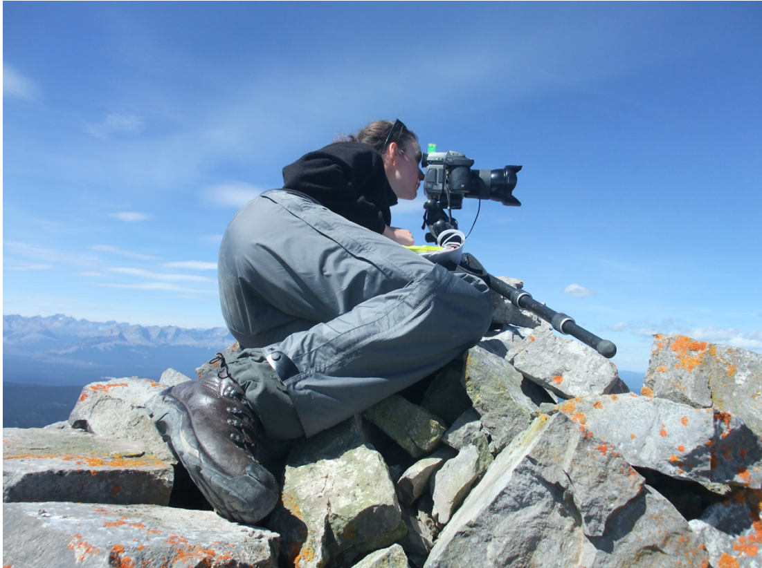
Figure 3-6. Tripod placement at Stn. 532 (Chungo). At times, the tripod must be placed on top of a cairn in order to achieve the perfect alignment; this example illustrates the capture of a repeat of Bridgland’s 1928 image. The station was visited during the 2014 field season, but is not part of the sample used in this study.
