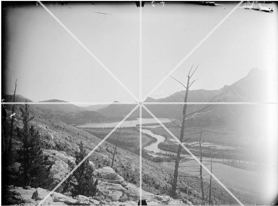
Figure 3-5. Landscape grid placed on a mastered image. Gridding is done using Photoshop prior to printing the image and taking it into the field. The grid on the photograph approximates that found on the camera viewfinder, thereby enabling more precise alignment of the repeat.
