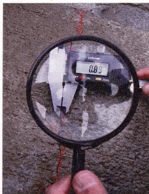
Figure 4.34 - Method of Measurement for Crack Widths, October 2003
