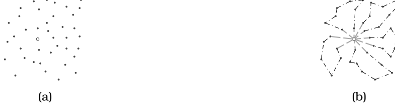
Figure 2.3: A CVRP example with n = 40 and k = 5 . Given the dispersed points shown in (a), CVRP asks to find the routes presented in (b).
