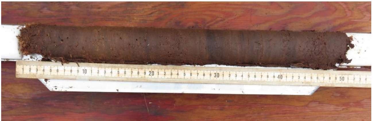
Figure 11: One of the 50-cm peat sections (70-120 cm) collected from Anderson Fen. (Photo by T. Lacourse)
