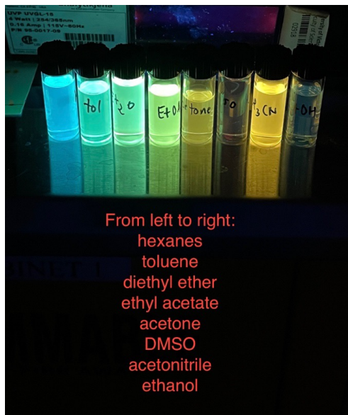
Figure 3-4. 2.14 illuminated with UV light displaying solvatochromic fluorescence.
