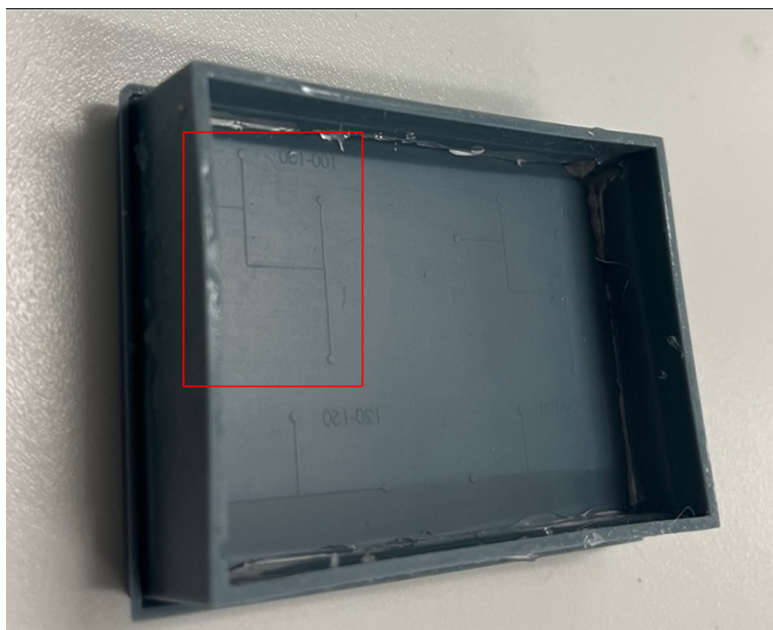
Figure 11: Completed resin mold
