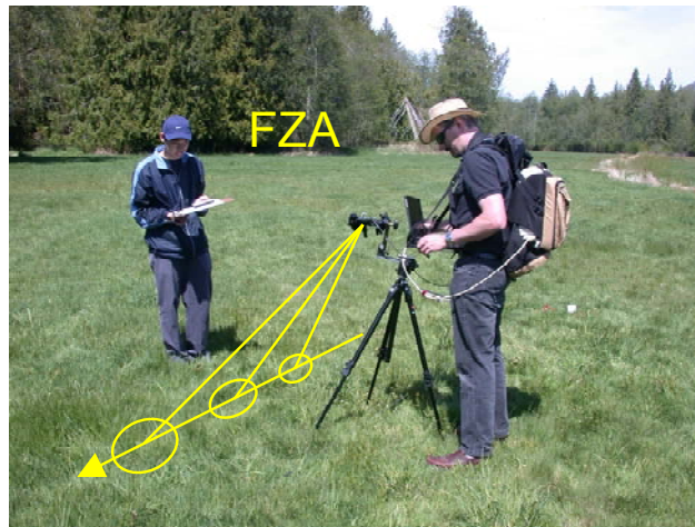
Figure 19. Setting up the simple goniometric system. FZA emulated by rotating the ASD along the flight path.
