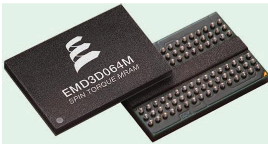
Figure 9. An Everspin spin-transfer-torque based magnetic random access memory chip for caching application. Reproduced with permission from [80], Copyright IEEE, 2014.
