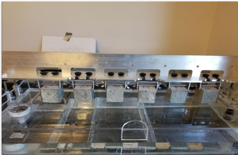
Figure 11: Testing the samples to obtain water absorption coefficient
