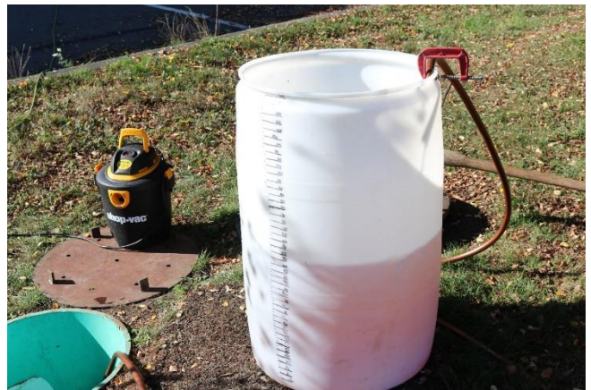
Photo 6. Effluent water pumping into small graduated tank.
