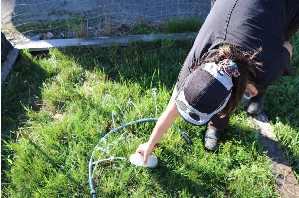
Photo 4. Perforated hose and TSS being applied to the cells.
