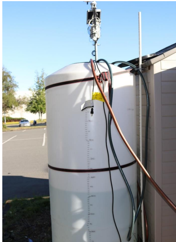
Photo 3. Graduated tank used to measure test volumes and mix nutrient pollutants.
