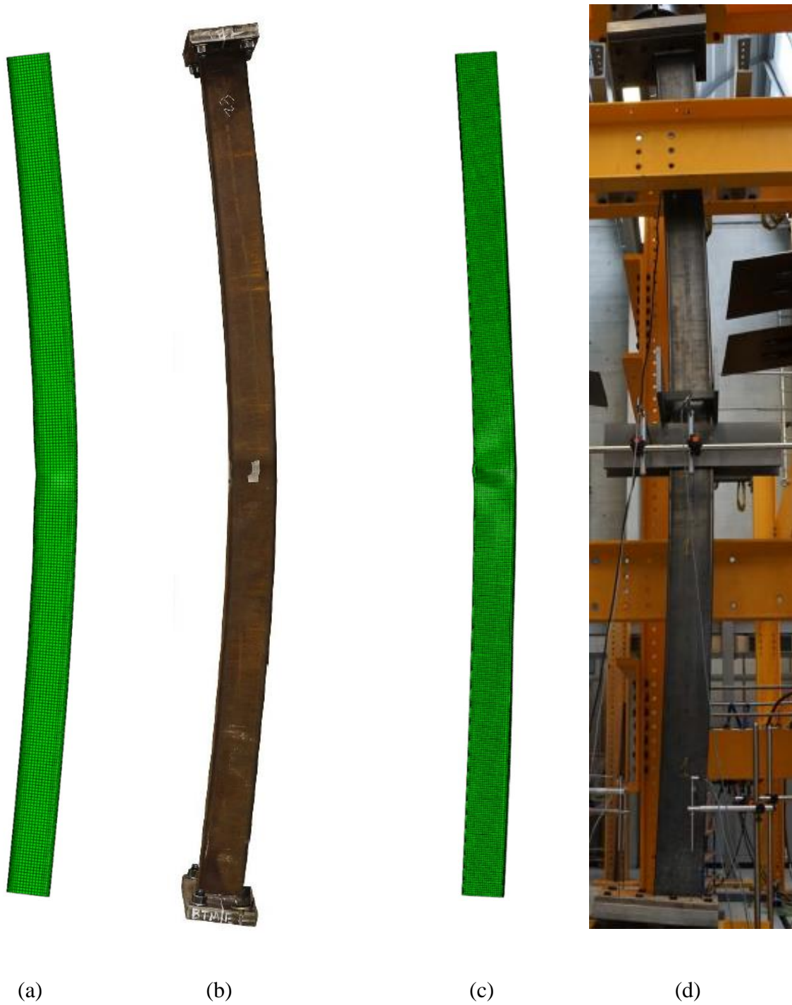
Figure 2.3 Comparison of the failure pattern between the FE model and test specimen: (a) SHS-IH-80×80×4-e40 FE model; (b) SHS-IH-80×80×4-e40 Test specimen [31, 32] (c) RHS-IN2-200×100×4-e85 FE model; (d) RHS-IN2-200×100×4-e85 Test specimen [26, 27]
